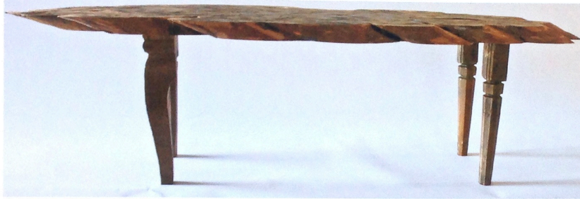
Top of slab brushed with angle grinder and burned with butane torch
