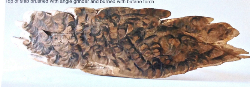
Top of slab brushed with angle grinder and burned with butane torch
